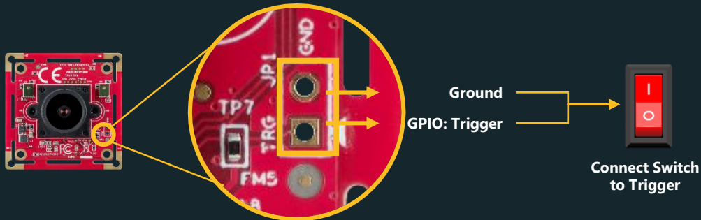
EV2U-SSM1-RLCF USB 2.0 2M @ 30 FPS External Trigger Low light
