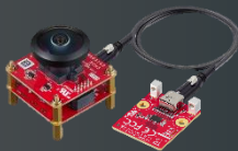
EV2C-GOM1 MIPI over Type-C 2M@ 30 FPS Fisheye
